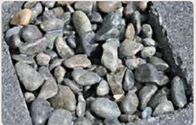
Notice how the Aquabind coats the surface of the pebbles and adheres them together. In this picture not quite dried yet.
