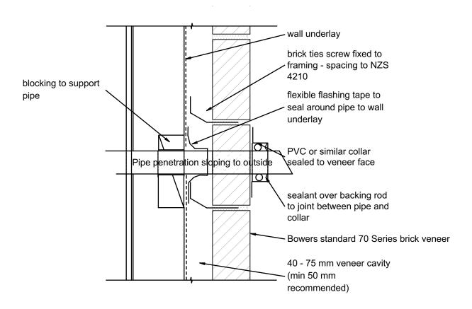
Penetrations - pipes up to 150 mm diameter (protected location)
