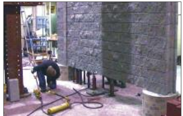
Assembled block wall with hydraulic jacks under the panel span for uplift test.
