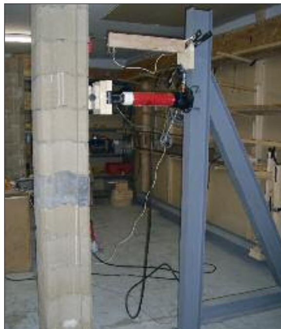
Hydraulic ram and frame assembly for AB Fence Post flexural test.
