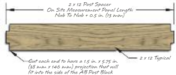
Figure 4: Post Spacer Jig
