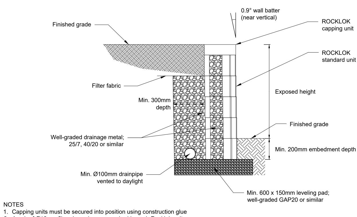
2. A pair of Ø16mm fibreglass pins are required in each Rocklok unit
