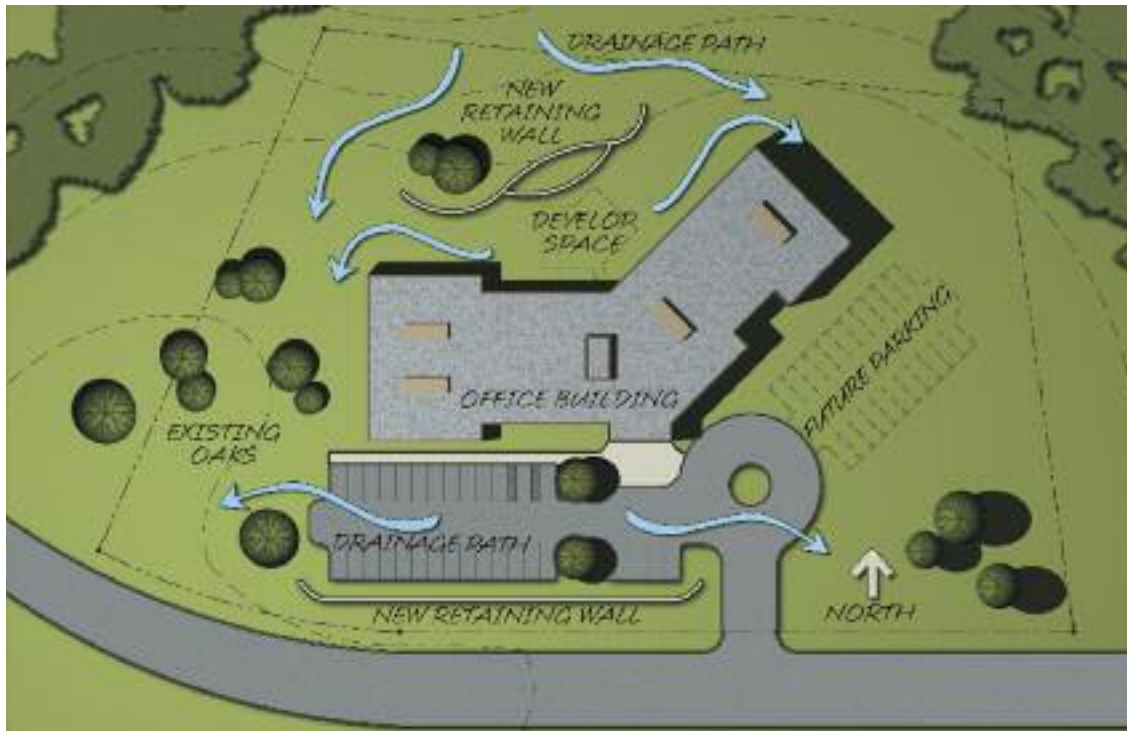
Note the site geometry above and below the proposed wall location.
