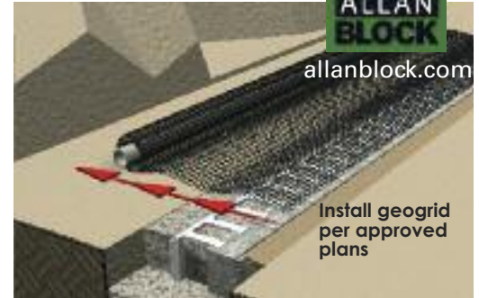
Install geogrid. Start in the middle of the facing unit and extend behind wall.
