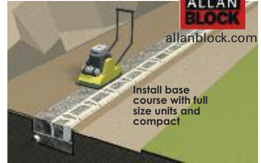
Install base course and compact.
